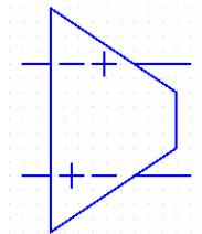
$$v_{id} = v_i^+ - v_i^-$$
