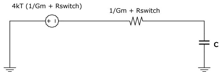
$$\overline{v_{oT}^2} = \frac{kT}{C} \left( 1 + \frac{R_{noise}}{R_{switch}} \right)$$
