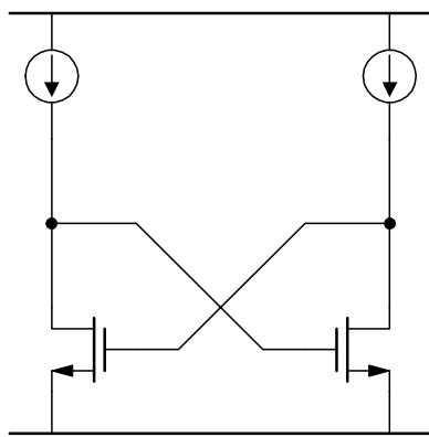
$$T_d = \frac{C}{g_m} \ln \frac{V_{od}}{V_{id}}$$
