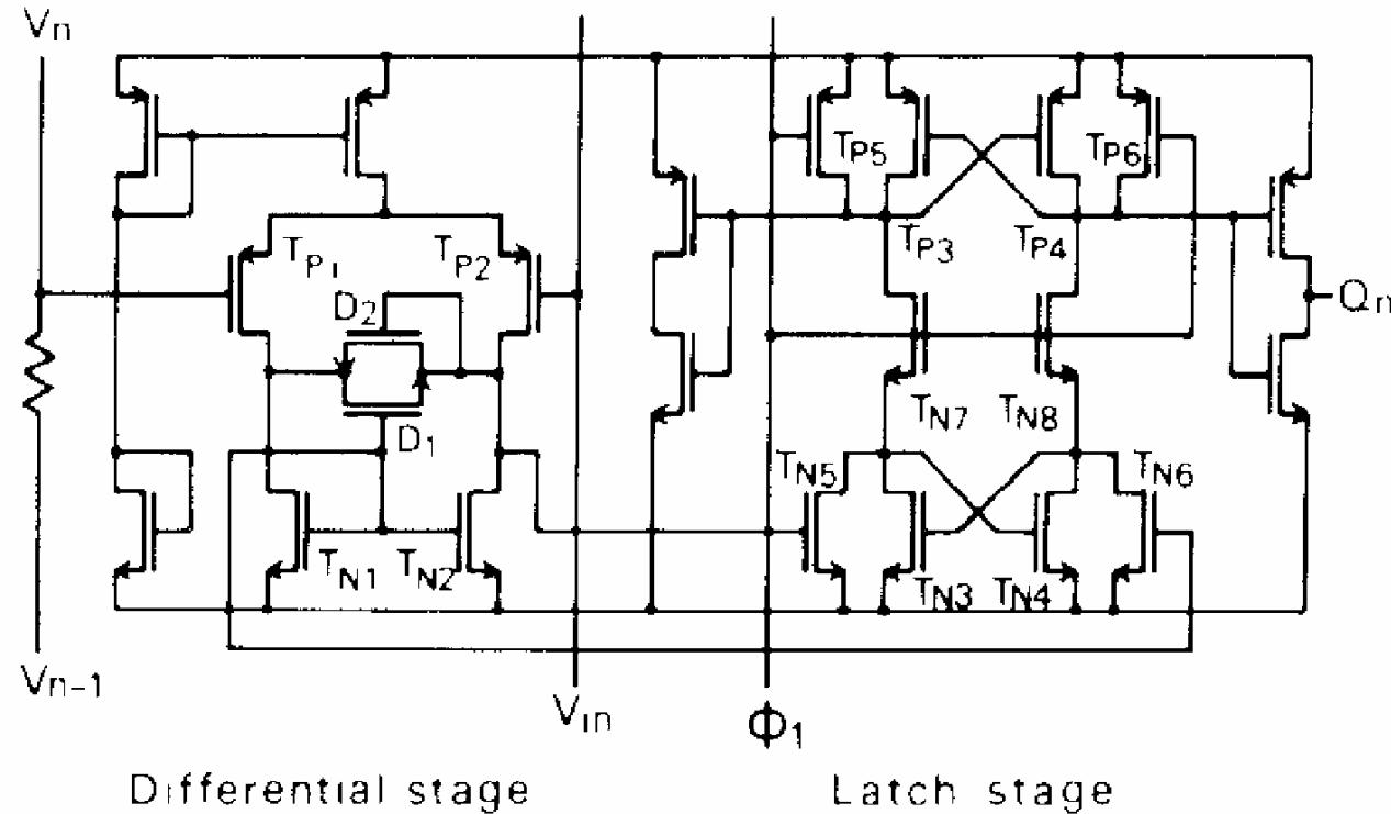
A. Yukawa, "A CMOS 8-Bit High-Speed A/D Converter IC," JSSC June 1985, pp. 775-9.
