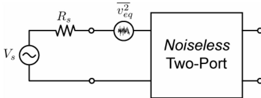
$$\overline{v_{eq}^2} = \overline{v_n^2} + \overline{i_n^2} R_s^2$$
