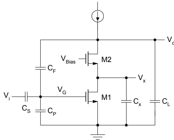
$$v_o = -\frac{1}{Fg_{m1}} \left( i_{n1} + i_{n2} \frac{s}{\omega_p} \right) \frac{1}{1 + \frac{s}{\omega_o Q} + \frac{s^2}{\omega_o^2}}$$
