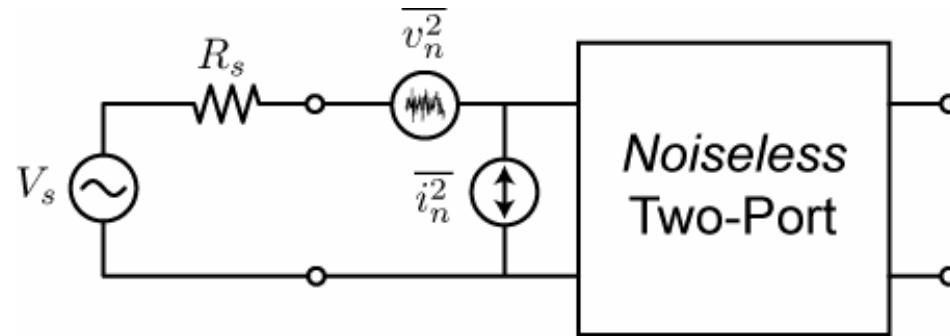
$$\begin{aligned}\overline{v_o^2} &= (\overline{v_n^2} A_v^2 + \overline{v_{R_s}^2} A_v^2) \left( \frac{R_{in}}{R_{in} + R_s} \right)^2 + \left( \frac{R_{in}}{R_{in} + R_s} \right)^2 R_s^2 \overline{i_n^2} A_v^2 \\ &= (\overline{v_n^2} + \overline{i_n^2} R_s^2 + \overline{v_{R_s}^2}) \left( \frac{R_{in}}{R_{in} + R_s} \right)^2 A_v^2\end{aligned}$$
