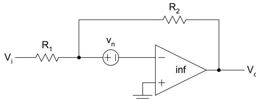
$$v_o = -v_i \underbrace{\frac{R_2}{R_1}}_{-A_{v0}} + v_n \frac{R_1 + R_2}{R_1}$$
