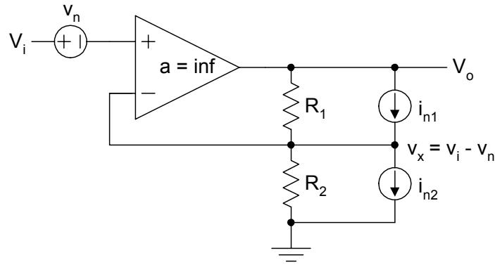
$$\begin{aligned}v_o &= R_1 \left( \frac{v_x}{R_2} - i_{n1} + i_{n2} \right) + v_x \\&= v_x \left( 1 + \frac{R_1}{R_2} \right) - (i_{n1} - i_{n2}) R_1 \\v_{ieq}^2 &= v_n^2 + (i_{n1}^2 + i_{n2}^2) \left( \frac{R_1 R_2}{R_1 + R_2} \right)^2 \\&\approx v_n^2 + \underbrace{4k_B T R_o \Delta f}_{v_{nfb}^2}\end{aligned}$$
