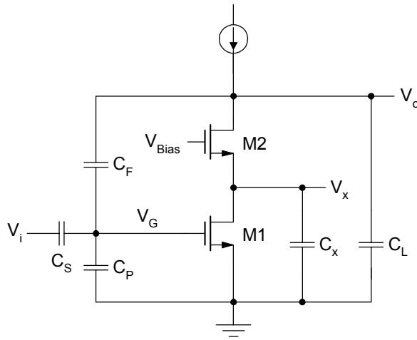
$$\frac{\overline{v_{on}^2}}{\Delta f} = \frac{4k_b T}{F^2 g_{m1}} \left( \underbrace{\frac{1}{M1} + \underbrace{\frac{g_{m2}}{g_{m1}} \left| \frac{s}{\omega_p} \right|^2}_{M2}}_{\left| \frac{1}{M1} + \frac{g_{m2}}{g_{m1}} \left| \frac{s}{\omega_p} \right|^2 \right|} \right) \left| \frac{1}{1 + \frac{s}{\omega_o Q} + \frac{s^2}{\omega_o^2}} \right|^2$$
