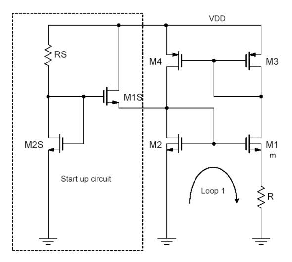
Startup circut: This one is very simple but the tradeoff is that it may be hard to turn off M1S completely, especially for low VDD.
