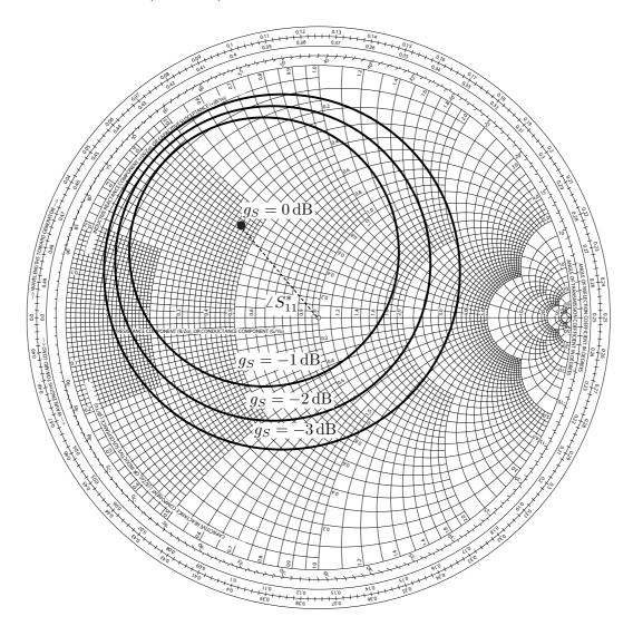
All gain circles lie on the line given by the angle of  $S_{ii}^*$ . We can select any desired value of source/load reflection coefficient to acheive the desired gain. To minimize the impedance mismatich, and thus maximize the bandwidth, we should select a point closes to the origin.
