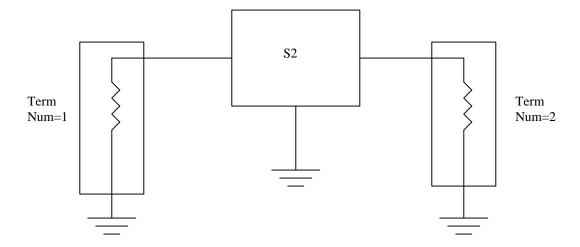
Your circuit must contain the S-parameter block that corresponds to the .S2P file created in Step 2. To create the S-parameter block, do the following:
