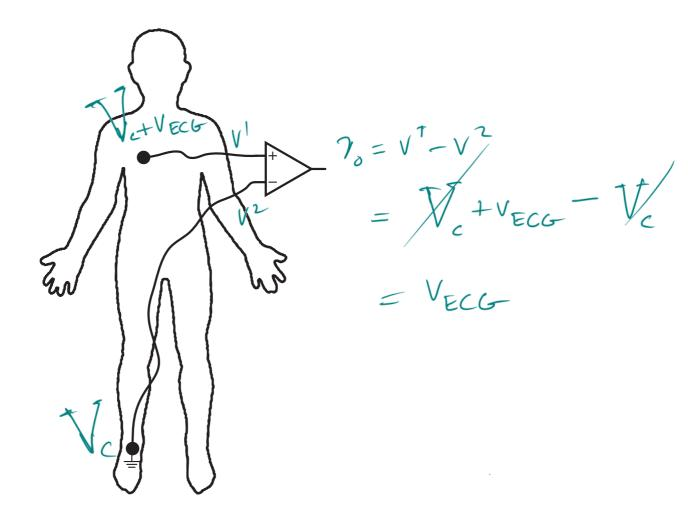
We thus need an amplifier that can detect a small differential mode voltage in the presence of a potentially very strong common mode voltage.
