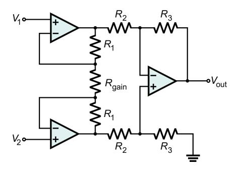
$$v_o = \left(1 + \frac{2R_1}{R_{gain}}\right) \frac{R_3}{R_2} (v_2 - v_1)$$
