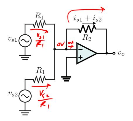
Each source is converted into a current and then summed in a similar fashion as the currents. Note that the virtual ground means that no current is "lost" when the currents are put in parallel (due to the output resistance).
