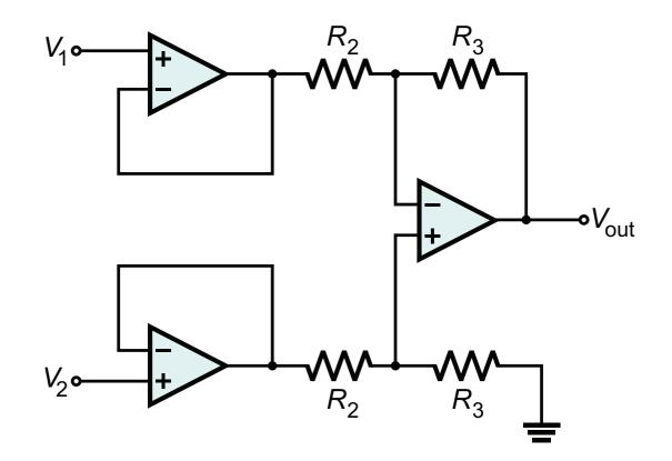
• Two unity-gain buffers are used to buffer the input signal. A difference amplifier is used to provide a gain of  $R_3/R_2$ .
