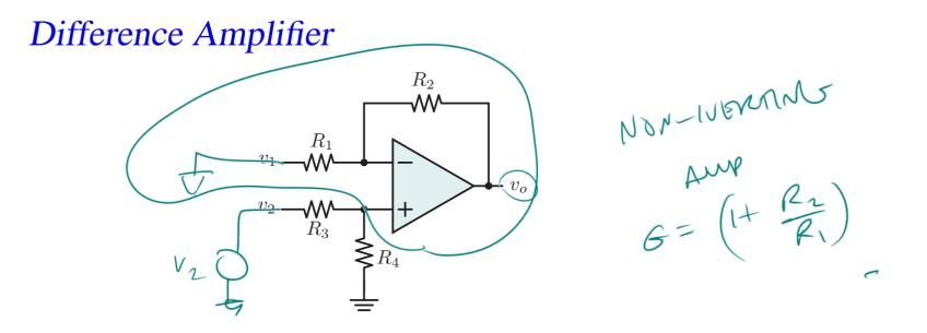
Using superposition, we can quickly calculate the transfer function. For port 1, the amplifier is simply an inverting stage  $V_2 = OV$
