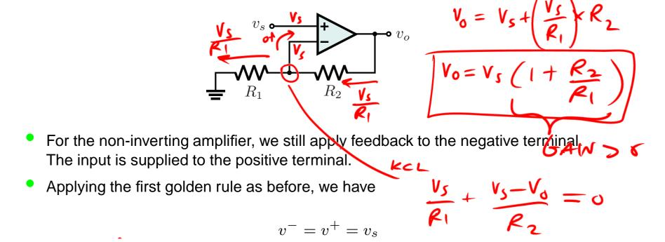
Now applying the second golden rule, since the input current of the op-amp is zero, there is a perfect voltage divider from the output of the op-amp to the negative terminal
