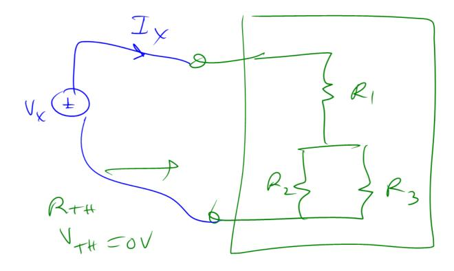
$R_{TH} = \frac{V_{X}}{I_{X}}$
