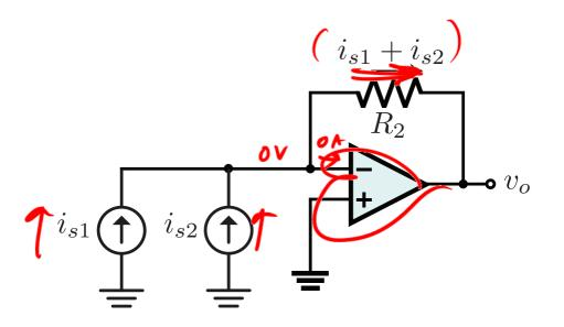
• An important observation is that in the inverting amplifier, the current injected into the negative terminal of the op-amp is routed to the output and converted into a voltage through  $R_2$ . If multiple currents are injected, then the *sum* of the currents is converted to a voltage.
