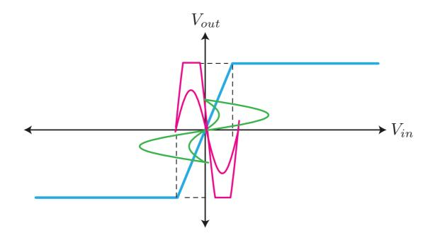
When the input signal goes beyond the linear range, the output can exhibit clipping, which is very non-linear.
