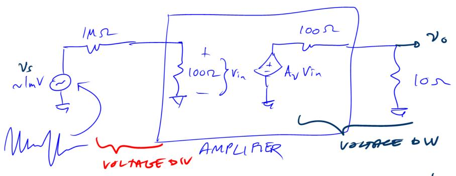
$$\gamma_{in} = \frac{100n}{100n + (Mn)} \gamma_s = \frac{100n}{1Mn} \gamma_s = 10^2 \times 10^6 \text{ Vs}$$
