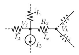
• Since the potential at the ground node is known, only n-1 unknown node voltages remain. Writing KCL at each other node results in an equation in the following form
