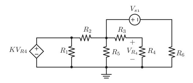
This example involves a dependent voltage source. The solution procedure is nearly identical to the case without the dependent source, except that we write the auxiliary equation to eliminate the additional unknowns.
