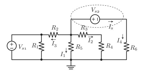
But note that if we write the KCL equations for both terminals of the voltage source, this unknown current appears twice.
