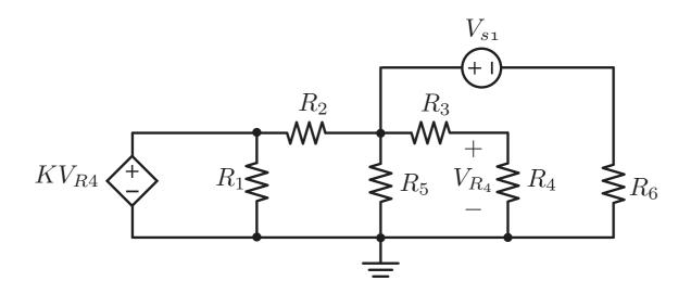
Nodes with dependent voltage sources are handled in the same way. They can also form supernodes and a KCL equation can be written for the supernode, just like independent sources. The only difference is that the potential difference between the floating dependent voltage source is not known until all the equations are solved.
