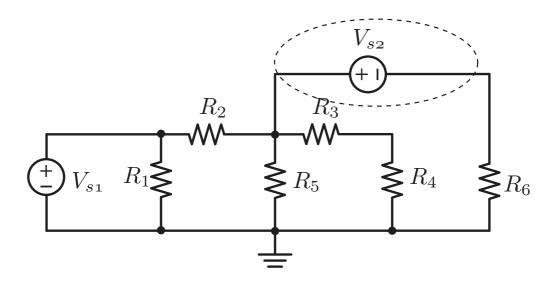
Using the steps that we have learned, we first identify a ground node at a convenient location (negative terminal of a source). Then we identify two super nodes in the circuit. For each super node we write KCL, put the equation into standard form, and solve.
