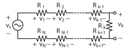
The equations for voltage divider and current divider are easy to generalize to Nseries or parallel resistors
