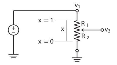
• For the circuit shown, since the total resistance is fixed, we can write
