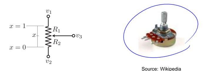
A variable resistor is called a rheostat. A related element has three terminals and it's called a potentiometer. It's typically constructed so that it presents a fixed resistance R across two of its terminals. The third terminal is connected to a point between the two other terminals in such a way that the resistance R<sub>2</sub> varies linearly (or perhaps logarithmically depending on the application).
