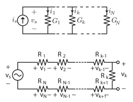
The equations for voltage divider and current divider are easy to generalize to N series or parallel resistors
