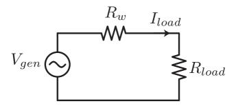
Say a house is dissipating  $P=1.2 {\rm kW}$  of power. If the house operated from a 120V DC source, then that's a current draw of (note we're ignoring the fact that most power delivered is AC rather than DC, but as we'll learn later, that's a simple correction factor)
