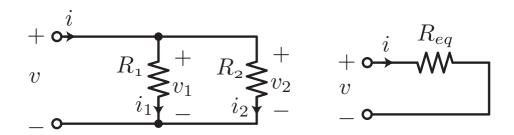
Shunt resistors are the "dual" of series resistors if we consider the conductance of the circuit. From KVL we know that the voltage across the shunt (parallel) components is equal
