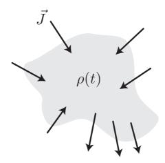
We know from fundamental physics that charge is conserved. That means that if in a given region the charge is changing in time, it must be due the net flow of current into that region. This is expressed by the current continuity relation in physics (which can be derived from Maxwell's equations)
