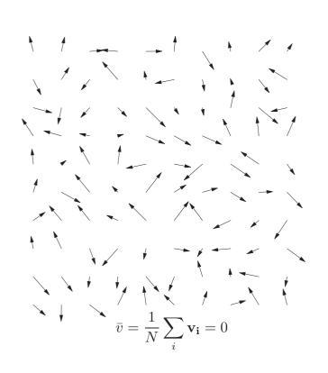
• The above result emphasizes that current is associated with motion. In our simple example, we assumed all carriers move at a velocity v. In reality, as you may know, electrons move very rapidly in random directions due to thermal motion  $(mv^2 \sim kT)$  and v is the net *drift velocity*.
