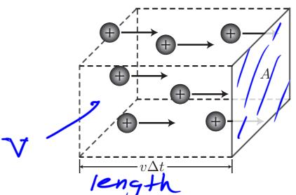
Suppose that the charge carriers each have a charge of q. Let's count the number of charges (c) crossing a surface in time  $\Delta t$  and multiply by the electrical charge
