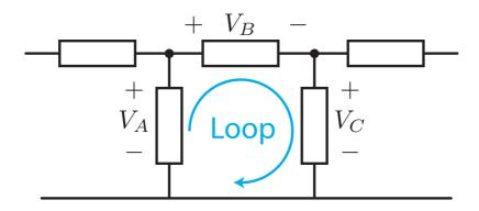
KVL states that the net potential around any loop in a circuit is zero
