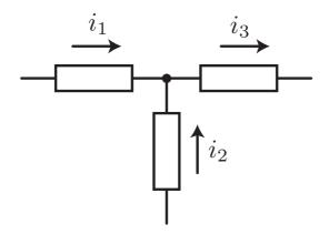
KCL states that the net charge flowing into any node of a circuit is identically zero.
