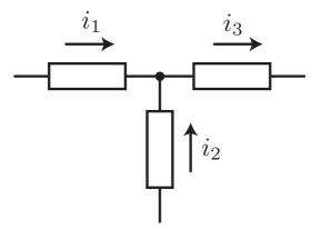
KCL states that the net charge flowing into any node of a circuit is identically zero. In the example shown
