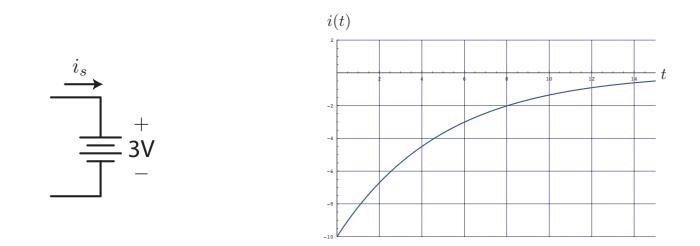
• Suppose a 3V voltage source has an instantaneous current of  $i_s(t) = -10e^{-t/5ns}$  mA, as shown above for t > 0. Find the net energy supplied by the source.
