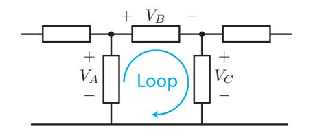
KVL states that the net potential around any loop in a circuit is zero
