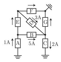
11. Use KVL to find the values of  $v_b$ ,  $v_c$ , and  $v_e$  for the circuit shown below. Which elements are connected in shunt?
