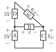
12. Use KVL to find the values of  $V_B$ ,  $V_D$ ,  $V_E$  and  $V_F$  for the circuit shown below. Which elements are connected in shunt?
