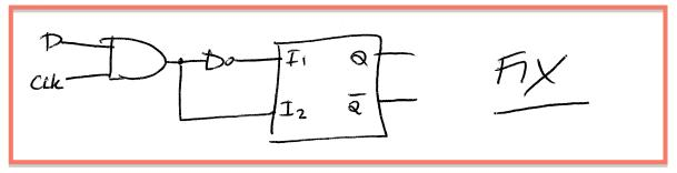
(c) (4 points) Design a positive edge triggered flip-flop using the D latch as a building block.
