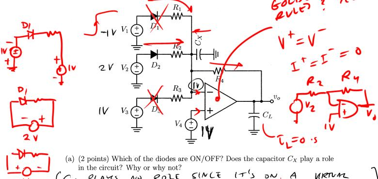
(b) (5 points) Use superposition to calculate the  $V_o$  as a function of  $V_1$ ,  $V_2$ ,  $V_3$ , and  $V_4$ .
