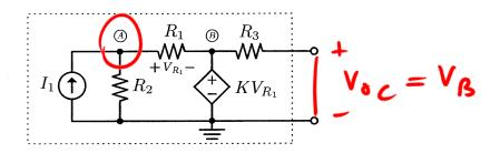
(a) (5 points) Find the open circuit voltage  $V_{oc}$  using KVL. Setup the node equations by using the nodes A and B as shown.
