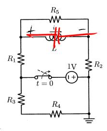
(a) (5 points) At time  $t = 0^-$ s, right before the switch opens, what's the inductor current  $i_L$ ?
