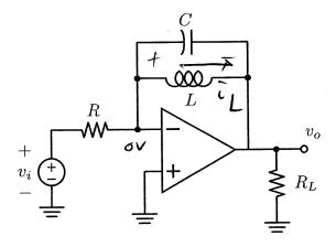
(a) (5 points) Write a differential equation describing the circuit behavior. Use  $i_L$  as the unknown quantity.
