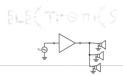
(c) (4 points) Calculate the voltage at the output driving the load speakers. Each speaker alone has an effective resistance of  $R_L = 9\Omega$ . The amplifier has an open-circuit voltage gain of 40dB ( $A_v = 100$ ) and an input resistance of  $10\Omega$  and an output impedance of  $3\Omega$ . Assume the source has a voltage of 1V.
