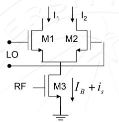
$$I_{o1} = I_1 - I_2 = F(V_{LO}(t), I_B + i_s)$$
