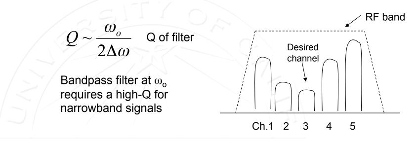
$\Delta f \sim 200 \text{ kHz} (\text{GSM})$
