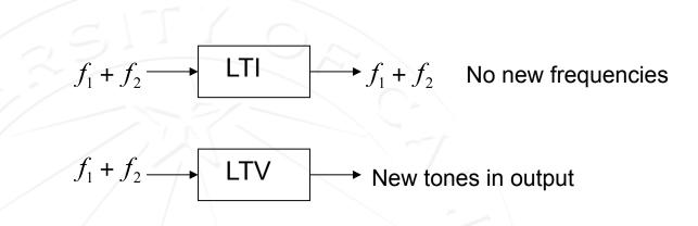
Example: Suppose the resistance of an element is modulated harmonically
