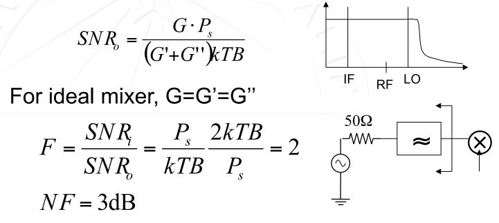
For a real mixer, noise from multiple sidebands can fold into IF frequency & degrade NF
