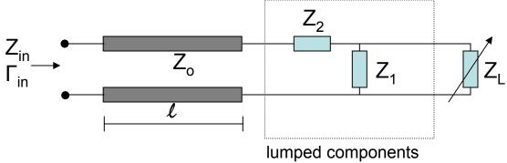
The lumped-components box has fixed impedances  $Z_1$  and  $Z_2$ .
