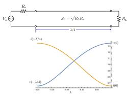
Note that a transmission line has the desired properties of voltage/current gain if there's a standing wave on the line.
