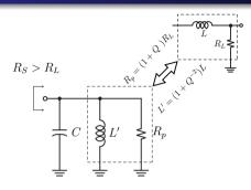
A quick way to accomplish this feat is to begin with the series to parallel transformation, where the load resistance in series with the inductor is converted to an equivalent parallel load equal to
