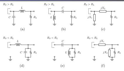
• Consider the *L*-Matching networks, named due to the topology of the network. We shall see that one direction of the *L*-match boosts the load impedance (in series with load) whereas the other lowers the load impedance (in shunt with the load).
