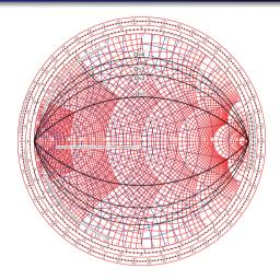
• For broadband matching, "hug" the x-axis. At high frequency, we can also include transmission line leads into the network.
