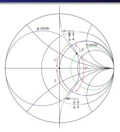
• Notice that there are two paths to get to the center. The difference is one is AC coupled versus DC coupled, so often the application will determine the choice.
