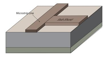
• Shunt stubs are easy but series stubs are not easy and require cuts in the ground plane.
