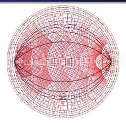
ullet Pick a desired Q (set by bandwidth), and then never allow the matching ratio to go above this value. The number of steps required will be set by the matching ratio.
