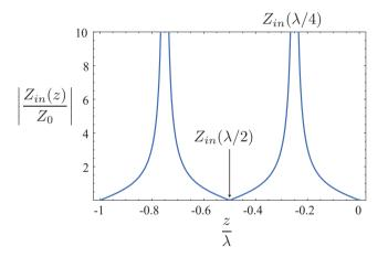
• The tangent function takes on infinite values when  $\beta \ell$  approaches  $\pi/2$  modulo  $2\pi$
