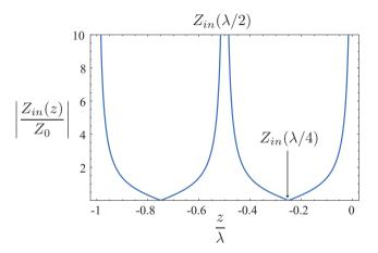
• The cotangent function takes on zero values when  $\beta\ell$  approaches  $\pi/2$  modulo  $2\pi$
