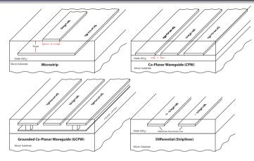
• If we restrict the structures to planar configurations, these are the most popular structures. The "Silicon Substrate" is partially conductive whereas on a PCB a non-conductive dielectric layer would be used. The conductivity of silicon leads to additional loss and higher order modes that should be suppressed.
