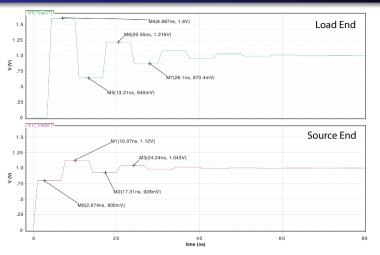
• Observed waveform as a function of time. Risetime due to SPICE  $t_{step} = 20 \text{ps}$ .
