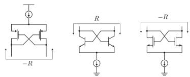
• The MOS or BJT cross coupled pair generate a negative resistance. Since  $i_x=i_{d2}=-i_{d1}$  and  $v_x=v_{gs2}-v_{gs1}$   $i_x=-G_mv_x=-\frac{g_m}{2}v_x$
