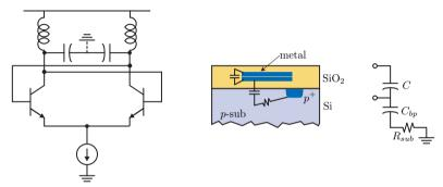
We can take advantage of virtual grounds in differential circuits. For instance, the bottom plate parasitics of MIM capacitors should be connected to the virtual grounds to avoid tank de-Qing.
