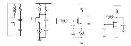
Single transistor MOS oscillator topologies are identical to the BJT versions shown last lecture. The large-signal properties of the oscillator, though, differ significantly due to the different current/voltage limiting mechanisms in MOS transistors.
