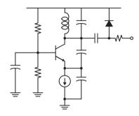
• The DC point of the varactor is isolated from the circuit with a capacitor. For a voltage  $V < V_{CC}$ , the capacitor is reverse biased (note the polarity of the varactor). If the varactor is flipped, then a voltage larger than  $V_{CC}$  is required to tune the circuit.
