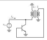
• Consider a test voltage source connected to the transistor
