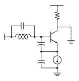
Note that the collector can be connected to a resistor without changing the oscillator characteristics. In fact, the transistor provides a buffered output for "free".
