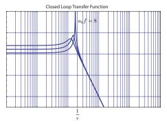
In the frequency domain perspective, we see that a feedback amplifier has a transfer function
