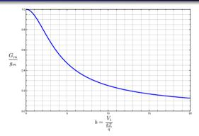
• For a differential pair (BJT), we can use numerical integration to find the ratio of the large signal  $G_m$  to the small-signal  $g_m$ . The *n*th harmonic (single-ended) output is given by:
