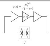
• As an example, consider a forward gain transfer function with three identical real negative poles with magnitude  $|\omega_p|=1/\tau$  and a frequency independent feedback factor f
