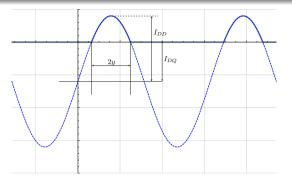
• Assume current pulses are sine wave tips, conduction angle is 2y
