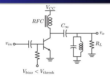
• Class C amplifiers are a wide family of amplifiers with conduction angle less than 180°. One way to achieve this is to bias a transistor below threshold and allow the input voltage to turn on the device for a small fraction of the cycle.
