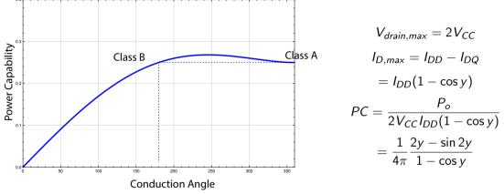
• The power capacity of Class C is low at low conduction angles. Peak is Class AB.
