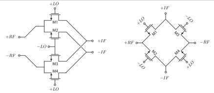
• Note that the Gilbert quad is really a folded ring. Thus the passive and active mixers are very similar. The main difference is how the quad devices are biased. In the Gilbert cell they are biased nominally in saturation and have DC current. In the passive mixers, they are biased near the threshold.
