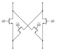
• A third way to draw the "ring" is as a butterfly switch. This representation clearly shows that the switching network, sometimes called a "butterfly" switch, will either connect the input to the output or invert the input and output.
