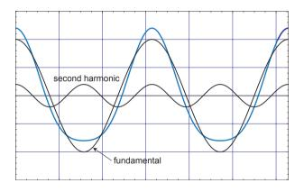
• The figure above demonstrates the waveform distortion due to second harmonic only.
