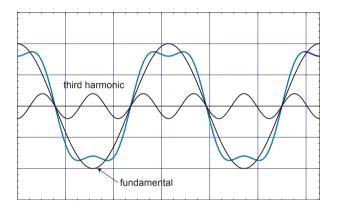
• The above figure shows the effects of the third harmonic, where we assume the third harmonic is in phase with the fundamental.
