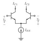
The differential pair is an important analog and RF building block.
