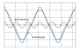
• The above figure shows the effects of the third harmonic, where we assume the third harmonic is out of phase with the fundamental.
