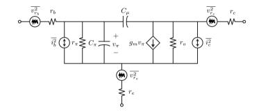
• The above equivalent circuit includes noise sources. Note that a small-signal equivalent circuit is appropriate because the noise perturbation is very small
