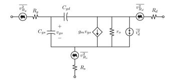
• The resistance of the substrate also generates thermal noise. In most circuits we will be concerned with the noise due to the channel  $\overline{i_d^2}$  and the input gate noise  $\overline{v_{R_a}^2}$
