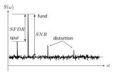
• The spurious free dynamic range *SFDR* measures the available dynamic range of a signal at a particular point in a system. For instance, in an amplifier the largest signal determines the distortion "noise" floor and the noise properties of the amplifier determine the "noise floor"
