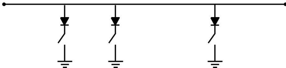
*Microwave modules use a transmission line shunted by PIN-diode switches in various combinations or use custom GaAs switches*
