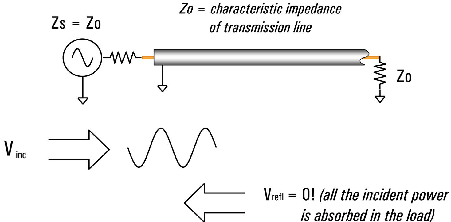
**For reflection, a transmission line terminated in  $Z_0$  behaves like an infinitely long transmission line**
