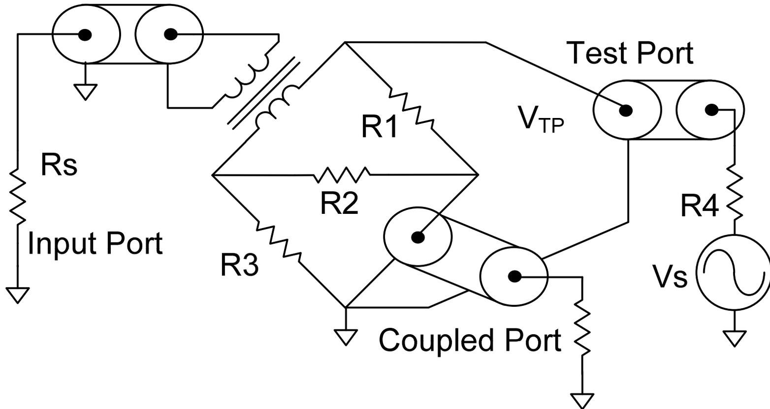
Just as clearly, with the signal driven from the test port, there will be the same loss to the Input Port as there was in the other direction, but now the signal will be coupled to the Coupled Port
