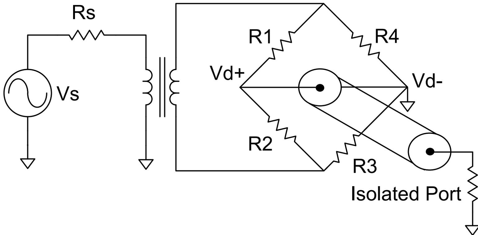
We would like the bridge to be matched so  $R_s^2 = R_1 \cdot R_3 = R_2 \cdot R_4$ .
