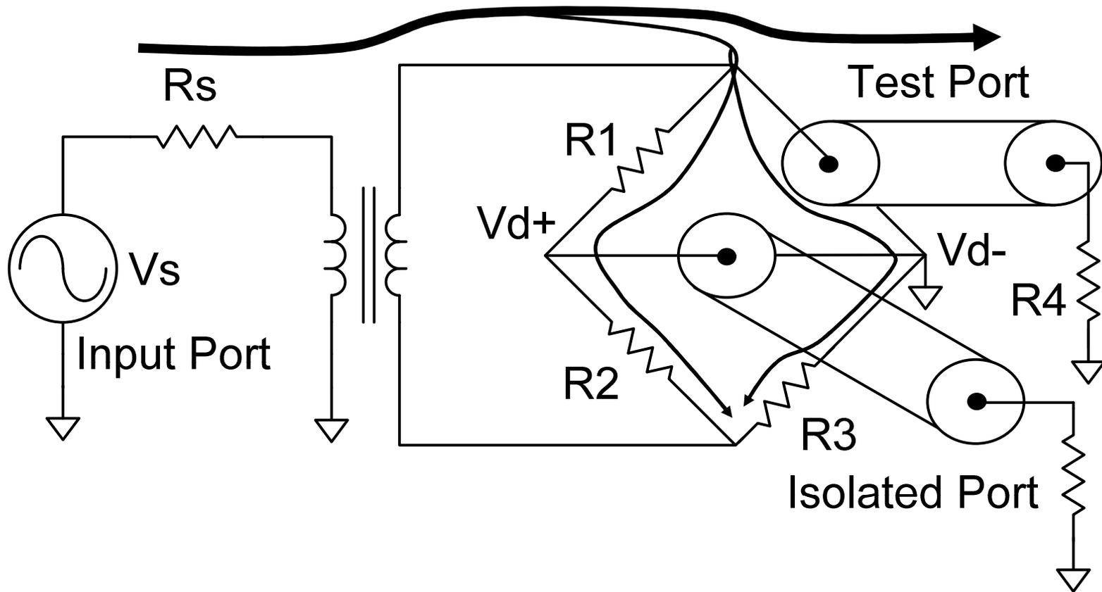
Now we can set the forward loss of the bridge. The voltage on the test port is equal to the voltage across R1. We have complete flexibility to set any ratio we want. In this case let's choose the voltage to be 5/6 of  $V_{in}$ . Then  $V_{d+} = V_{d-} = (1/6)V_{in}$ . The loss from Input Port to output port is  $20 \cdot \log(5/6) = -1.58$  dB.
