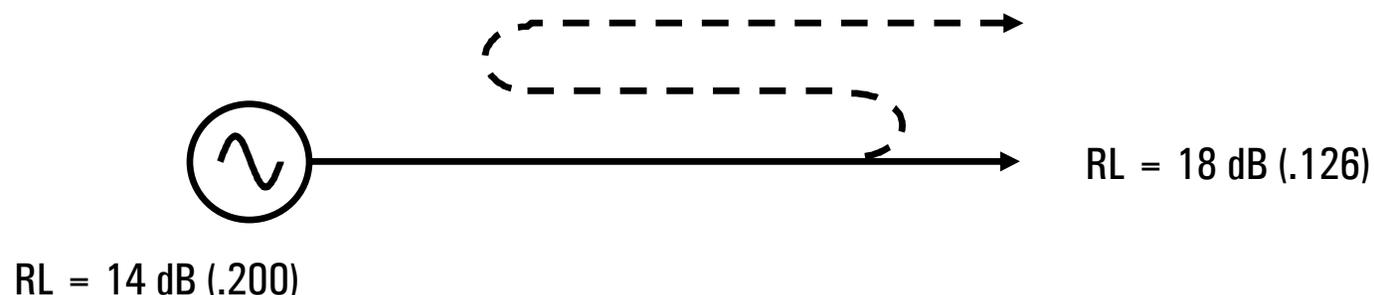
Thru calibration (normalization) builds error into measurement due to source and load match interaction
