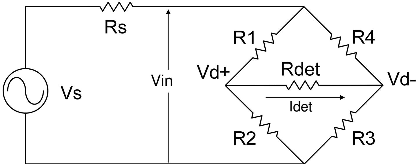
Further, it can be shown, that the input impedance of a balanced bridge follows the equation:  $Z_{in}^2 = R_1 \cdot R_3 = R_2 \cdot R_4$
