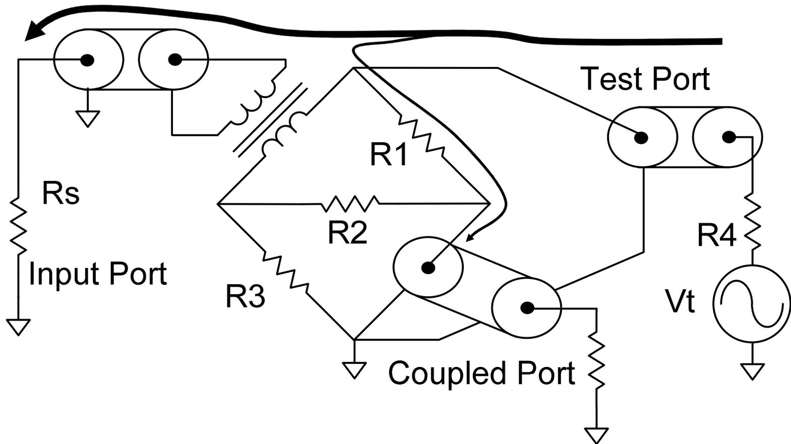
Let's check two cases: Assume the test port is open circuit ( $R_4$  infinite), then the voltage at the isolated point will be  $(1/2) \cdot (5/6) \cdot (1/6) \cdot V_s$ , exactly the same as the combination of loss and coupling, assuming a total reflection at the test port.
