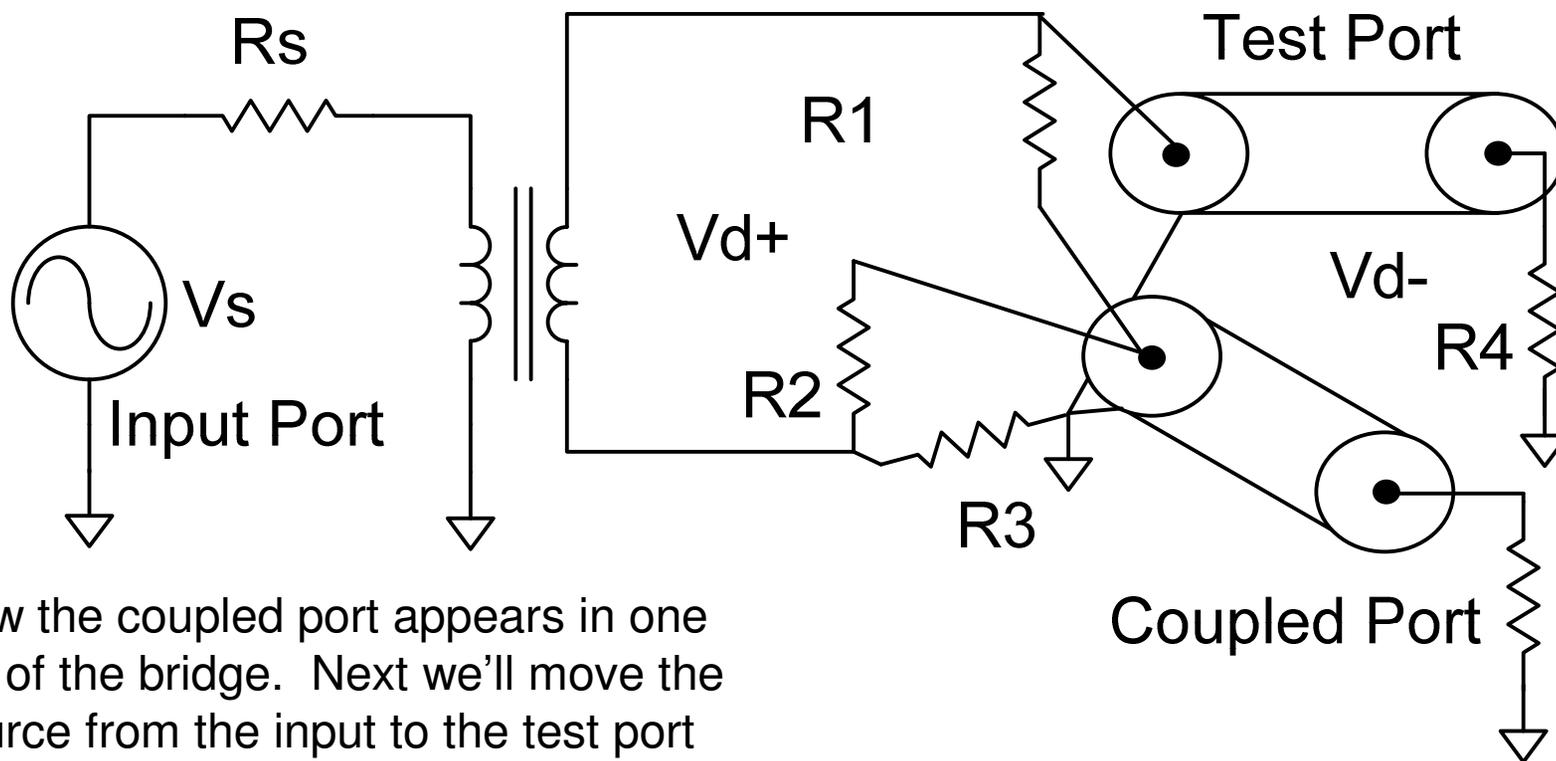
Now the coupled port appears in one leg of the bridge. Next we'll move the source from the input to the test port (and make the input into a port as well)
