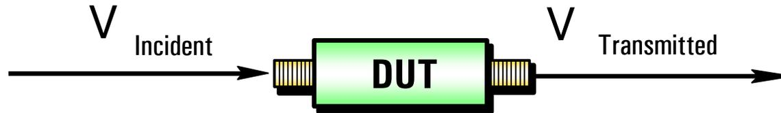
$$\text{Transmission Coefficient} = T = \frac{V_{\text{Transmitted}}}{V_{\text{Incident}}} = \tau \angle \phi$$
