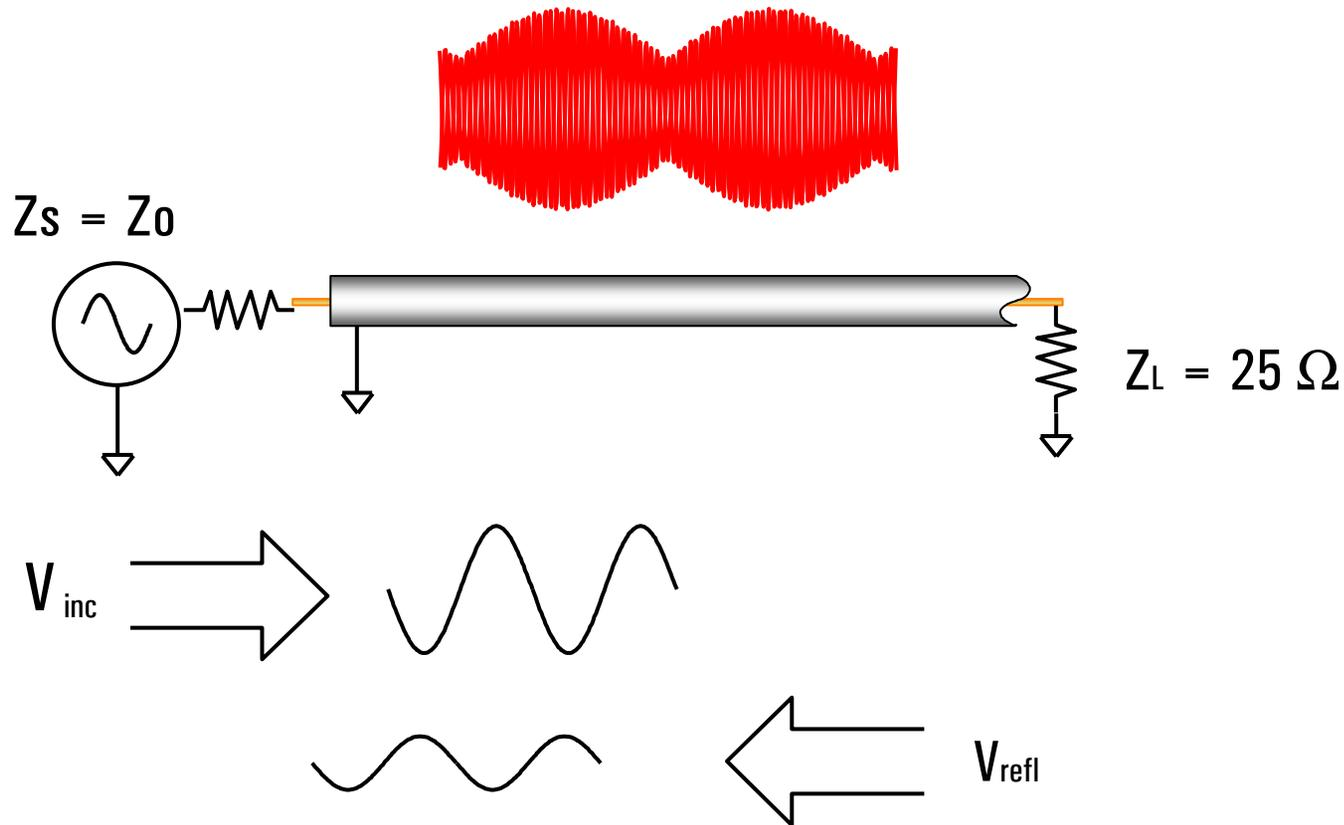
**Standing wave pattern does not go to zero as with short or open**
