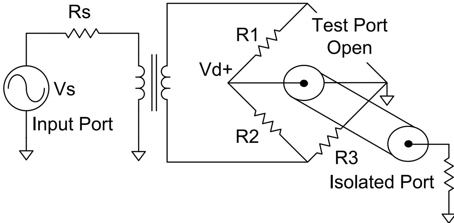
Now Assume the test port is short circuit ( $R_4 = 0$ ). Surprisingly (or not, if you're a real electrical engineer) the voltage at the isolated port will be  $(1/2) * (5/6) * (1/6) * V_s$ , exactly the same as the open, but with a sign change! Thus it is again the combination of loss and coupling, assuming a total reflection at the test port, but the reflection is negative.
