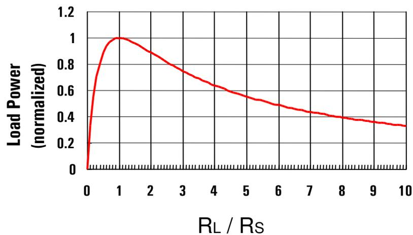
**Maximum power is transferred when  $R_L = R_S$**
