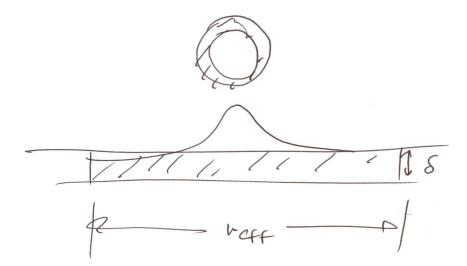
4. (10 points) Using the fact that a capacitor stores energy equal to  $\frac{1}{2}CV^2$ , and the electrostatic field has energy density of  $\frac{1}{2}\mathbf{E}\cdot\mathbf{D}$ , calculate the capacitance of the following structure by equating the total energy stored in the cap to the energy contained in the electrostatic field. Neglect fringing fields.
