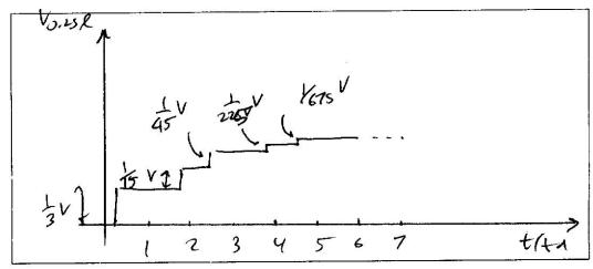
(d) Sketch the voltage waveform on the first transmission line at  $t = 3.5t_d$ .
