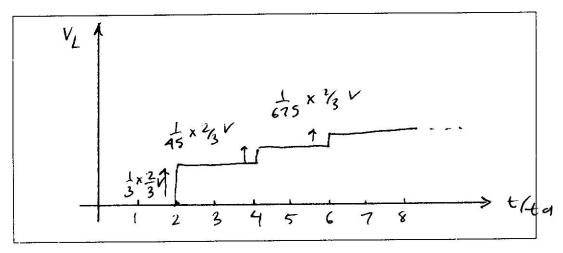
(c) Sketch the voltage waveform at the point  $z/\ell=.25$  as a function of time on the first transmission line.
