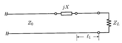
(a) Using the Smith Chart below, find  $\ell_1$  and X to perform an impedance match. It should be noted that the stub must be placed at ground level, in other words a distance of at least 100m from the load.
