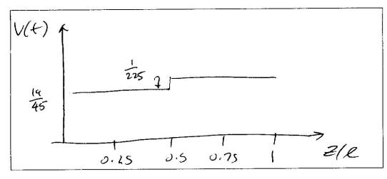
4. (20 points) The transmission line below has a discontinuity connected in shunt as shown below. The discontinuity consists of a capacitor and a parallel resistor. The load is matched to the line. Derive the equations governing the reflection  $v^-$  at the discontinuity.
