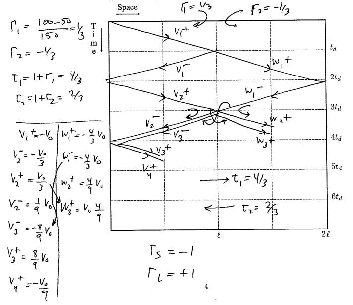
(b) Sketch the voltage waveform at the interface (versus time).
