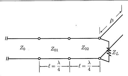
(b) Consider the matching circuit shown above where the load  $Z_L$  is transformed into  $Z_0 = 50~\Omega$ . Specify the component values  $Z_{02}$  and  $\ell_1$  to obtain an impedance match. ( $Z_{01} = 62~\Omega$  and  $Z_L = 27.455 + j50~\Omega$ ). The open stub of length  $\ell_1$  has an impedance of  $Z_0$ .
