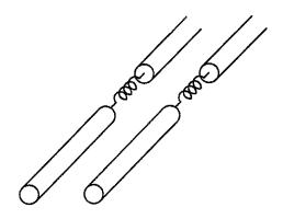
(e) In order to increase the communication distance further by a factor of 10, lumped inductors are periodically loaded onto the line as shown above. Specify the number and value of inductance needed to do this if the maximum allowed spacing between the inductors is  $\lambda/10$  and the communication frequency is 1 MHz. Explain why this works.
