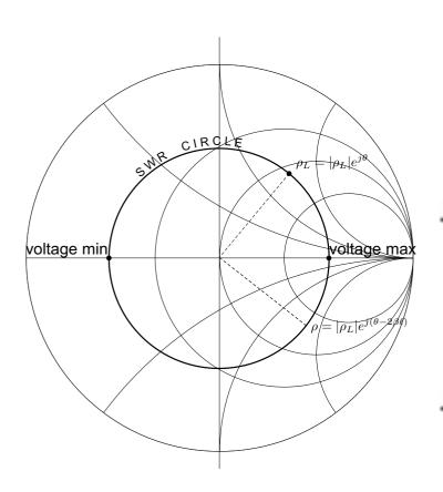
Recall the voltage max occurs when the reflected wave is in phase with the forward wave, so
