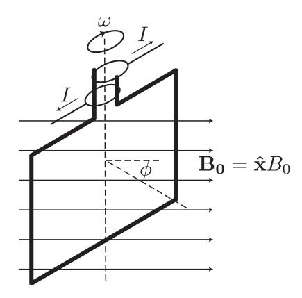
A simple AC motor/generator consists of a rotating loop cutting through a constant magnetic field. The slip rings maintain contact with the loop as it rotates.
