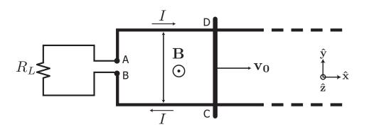
• Consider the following "generator". A bar of length  $\ell$  moves to the right with velocity  $v_0$  (always making contact with the rest of the circuit)
