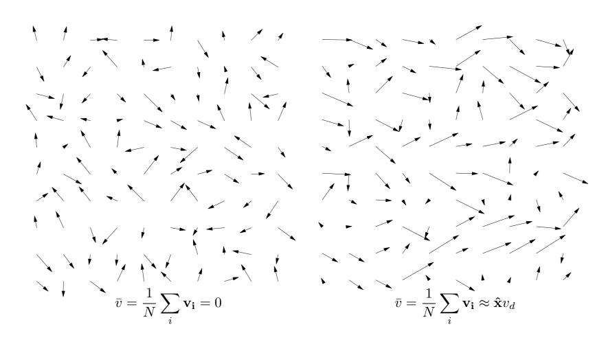
In the left figure, electrons are moving with random velocity (net motion is zero). On the right figure, electrons are moving with random velocity plus a drift component to the right (drift has been exaggerated).
