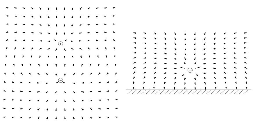
The vector field plot for a dipole distribution is shown on the left. The upper half field plot is also the solution to the monopole charge placed near a ground plane.
