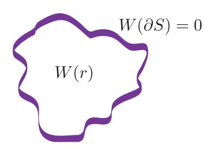
In particular, W(r) is the solution to the problem with zero boundary conditions. But if W is zero on the boundary and non-zero in the interior of the problem space, then clearly W must have maximum or minimum point. But such a function cannot be a solution to Laplace's equation.
