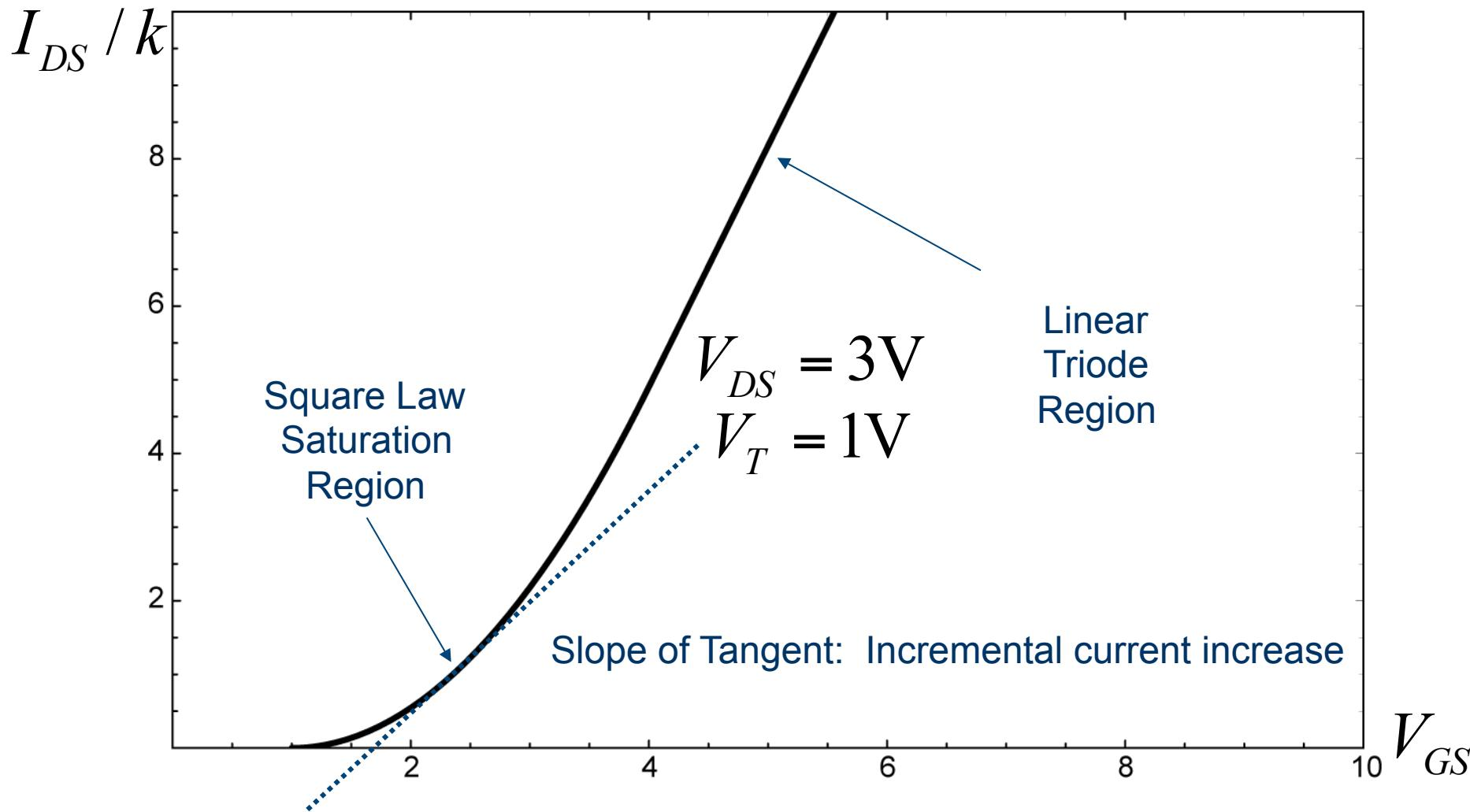
Assumption:  $V_{DS} > V_{DS,SAT} = V_{GS} - V_{Tn}$  (square law)
