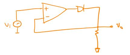
Use an op-amp to make the circuit precise.
