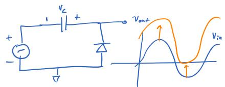
In this circuit the diode turns on initially and charges the capacitor to the AC voltage. Note that once the voltage starts to drop, the diode turns off.
