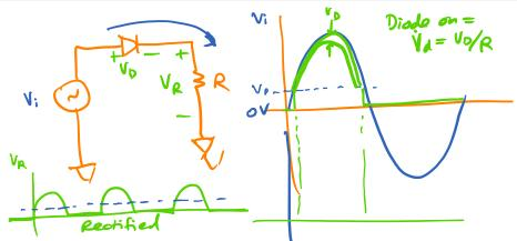
The simple circuit shown above will only conduct during the positive cycle of the sinusoidal voltage.
