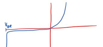
Note that by this argument, the leakage current is independent of the reverse bias. Electrons will 'float' up the barrier no matter the height! Holes will 'fall' down the barrier no matter the height.
