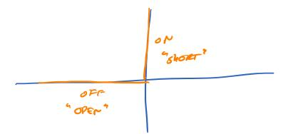
An ideal diode only allows current to flow in one direction. That's because the current is zero when a negative voltage is applied. When a positive voltage is applied, any current can flow and so the diode looks nearly like a short circuit. Can you give an argumetn for why this ideal diode cannot exist? *Hint:* Try a thermodynamic argument.
