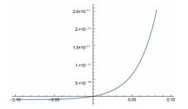
Even without a forward bias voltage, some small leakage current flows through the diode. This is because there are always a very small number of electrons (holes) in the p-type (n-type) material that are moving around. If they reach the potential barrier, they "float up" (remember they are electrons) or "fall" off the barrier. There are so few electrons (holes) in the p-type (n-type) material that this is a rare occurrence.
