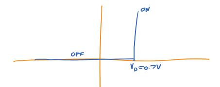
An ideal diode only allows durrent to flow in one direction. That's because the current is zero when a negative voltage is applied. When a positive voltage is applied, any current can flow and so the diode looks nearly like a short circuit. The "on" voltage is related to the required forward bias, which for Si is about 0.7V.
