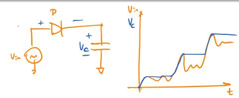
The capacitor is charged to the peak voltage and the output is held at the peak. Any excursions below peak cannot forward bias the capacitor. If a voltage excursion exceeds the peak up to a given point, then the capacitor is quicky charged by the forward biased diode.
