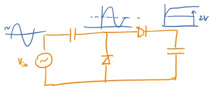
If we rectify the above voltages, we can generate positive or negative DC voltages of twice the magnitude. This is a voltage doubler!
