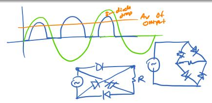
This bridge circuit will conduct current during both cycles. Due to the polarity of the diodes, current is always flowing in the same direction through the load, even for a negative voltage. This means that the circuit performs an absolute value function.
