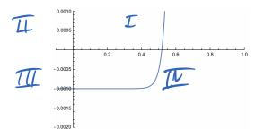
Note that a solar cell is equivalent to a forward biased diode in parallel with a current source.
