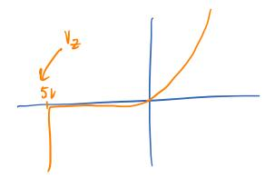
When breakdown occurs, the diode behaves like a battery. No matter what current is drawn, the voltage is nearly constant. This is often used as a voltage reference. The breakdown mechanism can be due to quantum mechanical tunneling or due to avolanch breakdown.
