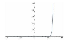
When a "forward-bias" is applied across the diode, lowering the built-in potential, a rush of current flows across the junction. It can be shown that this current is an exponential function of the barrier height.
