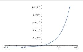
• Even without a forward bias voltage, some small leakage current flows through the diode. This is because there are always a very small number of electrons (holes) in the p-type (n-type) material that are moving around. If they reach the potential barrier, they "float up" (remember they are electrons) or "fall" off the barrier. There are so few electrons (holes) in the p-type (n-type) material that this is a rare occurrence.
