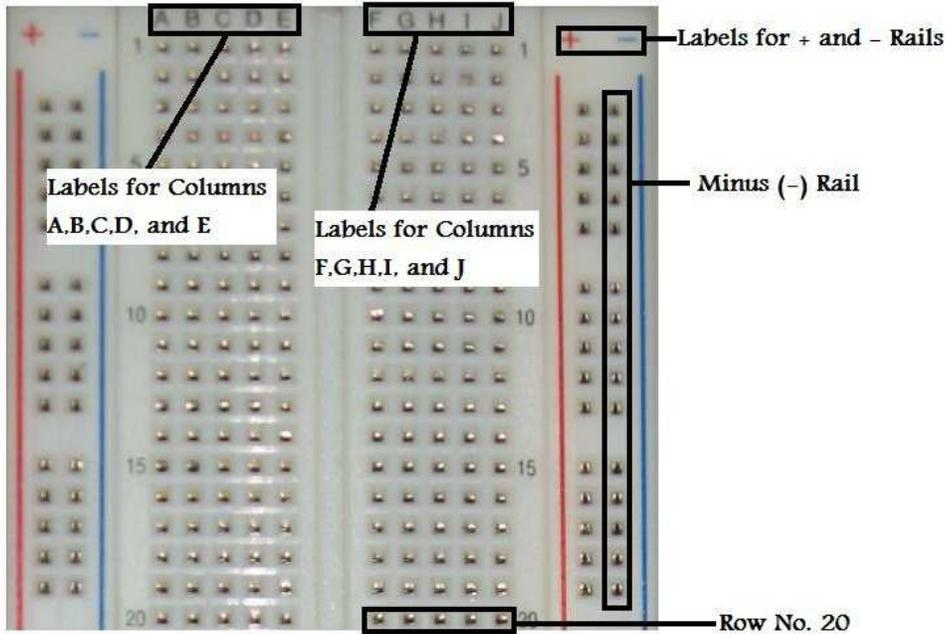
Figure 1: A typical breadboard
