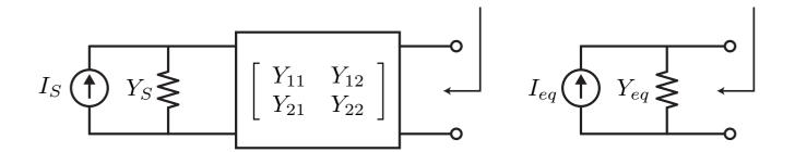
To derive the available power gain, consider a Norton equivalent for the two-port where
