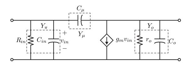
${\color{red} \bullet}$  Let's compute the Y parameters for the common hybrid-  $\!\Pi$  model
