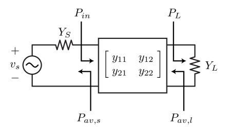
• We can define power gain in many different ways. The power gain  $G_p$  is defined as follows
