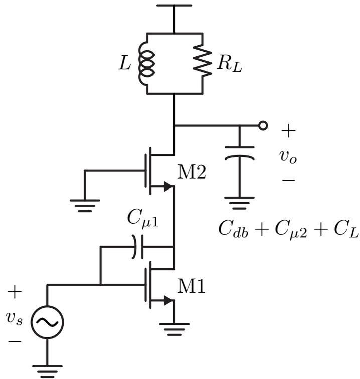
Besides the obvious advantage of boosting the output impedance, thus maximizing the  $Q$  of the load, the cascode device solves a major stability problem of the amplifier.
