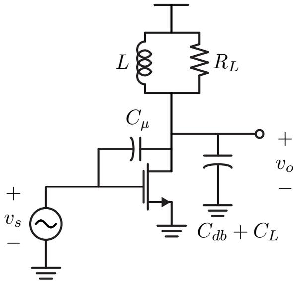
The  $RLC$  loaded amplifier is a tuned amplifier. A transconductance device drives a shunt  $RLC$  load which results in a voltage gain.
