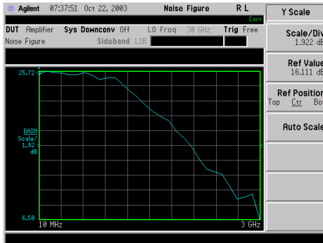
Figure 13: Full screen display of Noise figure and device gain
