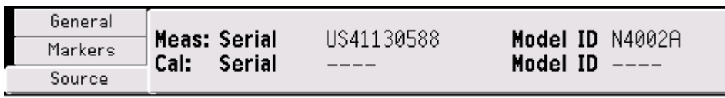
Figure 15: Noise source information: Cal information is blank because user selected common ENR table
