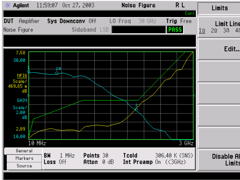
Figure 19: Measurement with limit test on, showing a passing noise figure limit test
