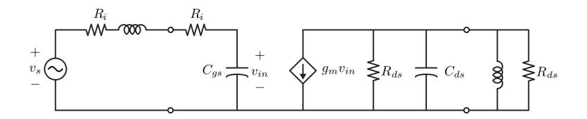
A more realistic equivalent circuit is shown above. If we make the unilateral assumption, then the input and output power can be easily calculated. Assume we conjugate match the input/output
