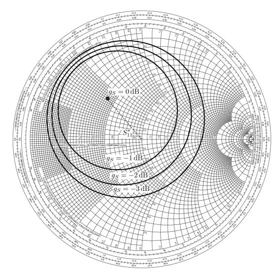
• All gain circles lie on the line given by the angle of  $S_{ii}^*$ . We can select any desired value of source/load reflection coefficient to acheive the desired gain. To minimize the impedance mismatch, and thus maximize the bandwidth, we should select a point closest to the origin.
