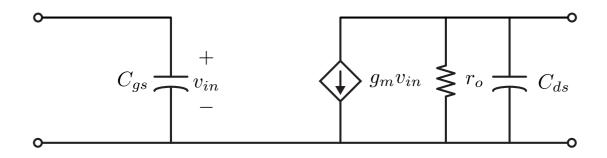
• The AC equivalent circuit for a MOSFET at low to moderate frequencies is shown above. Since  $|S_{11}| = 1$ , this circuit has infinite power gain. This is a trivial fact since the gate capacitance cannot dissipate power whereas the output can deliver real power to the load.
