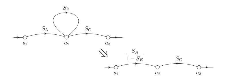
• Rule 3: (self-loop rule) We can remove a "self-loop" by multiplying branches feeding the node by  $1/(1 - S_B)$  since
