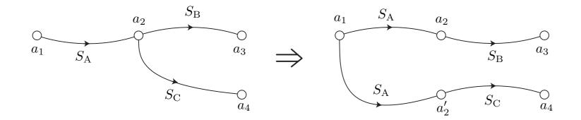
• We can duplicate node  $a_2$  by splitting the signals at an earlier phase
