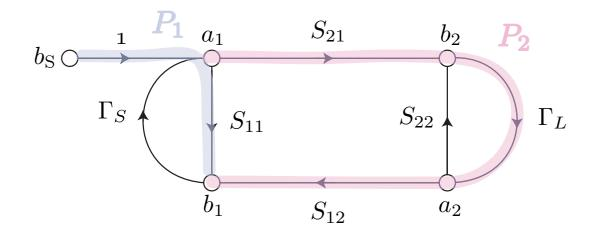
Using Mason's Rule, you can calculate the transfer function for a signal flow graph by "inspection"
