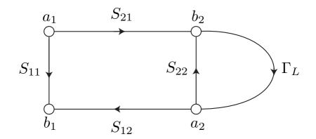
• Using Mason's rule, you can quickly identify the relevant paths for a  $\Gamma_{in} = b_1/a_1$ .
