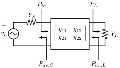
We can define power gain in many different ways. The power gain G<sub>p</sub> is defined as follows
