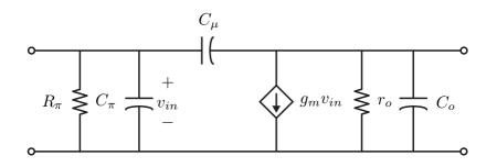
The hybrid-pi model for a transistor is shown above. Under what conditions is this two-port active? The hybrid matrix is given by
