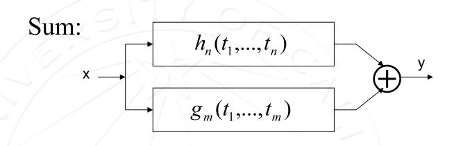
$$f_n(t_1, t_2, ..., t_n) = h_n(t_1, ..., t_n) + g_m(t_1, ..., t_m)$$
