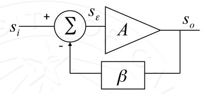
Let  $s_o = A_1(j\omega_a) \circ s_2 + A_2(j\omega_a, j\omega_b) \circ s_{\varepsilon}^2 + ...$  $s_{fb} = \beta(j\omega_a) \circ s_o$   $s_{\varepsilon} = s_i - s_{fb}$
