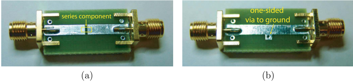
Figure 19: (a) Open and (b) short structures used for the automatic port extension feature of the network analyzer.
